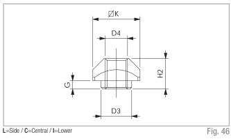
Steel nuts to be used in the slots of the body.
