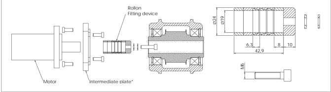
\* Any intermediate plate that may be necessary must be manufactured on site.
