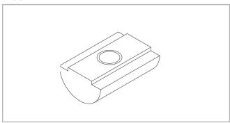
Steel nuts to be used in the slots of the body.
