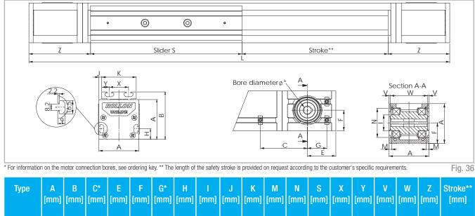
C75 75 90 71.5 53.5 38.8 34.5 20 Ø 29.5 5 65 4.85 Ø 55 285 36 14.5 2.3 70.4 116 3000 For the position of the T-nuts when using our motor adapter plates, see p. US-27ff Tab. 46 \*\* Maximum stroke for a single-piece guiding rail. For longer strokes, see tab. 51
