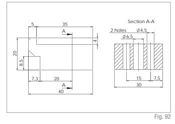
Fixing clamp (for all sizes except A100) for simple mounting of a linear axis on a mounting surface or for connecting two units with or without a connection plate (see p. US-70).
