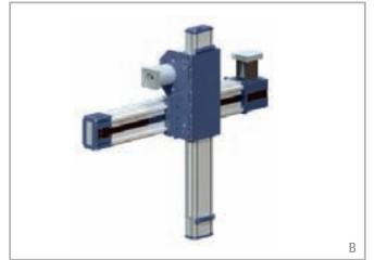
B - Linear units: X axis: 1 ROBOT 160 SP... Z axis: 1 SC 130Connection part: None
