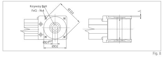
An (optional) connection flange is required to fit the standard reduction units selected by Rollon. For further information, contact our offices
