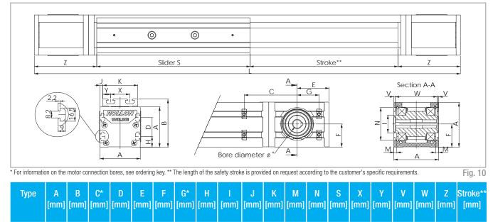
A75 75 90 71.5 35 53.5 38.8 34.5 20 Ø 29.5 5 65 4.85 Ø 55 285 36 14.5 2.3 70.4 116 For the position of the T-nuts when using our motor adapter plates, see p. US-15ff
