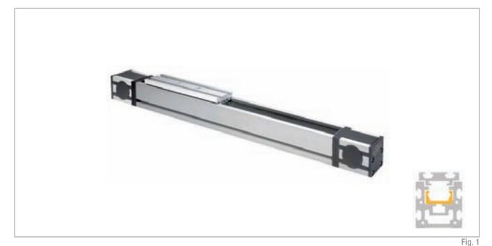
Uniline is a family of ready-to-install linear actuators. They consist of internal Compact Rail roller sliders and steel-reinforced polyurethane belts in a rigid aluminum profile. Longitudinal seals enclose the system. This arrangement provides the best protection for the actuator from soiling and damage. In the A series, the fixed bearing rail (T-rail) is mounted horizontally in the aluminum profile. Versions with long (L) or double (D) sliders in one axis are possible.
