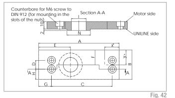
\* Area of plate needs to be cut if used for ED75 linear unit. (Adding 20 mm to total length of unit will render this modification unnecessary). Othewise it gets in contact with the outer rail. X = 20 mm; Y = 35 mm
