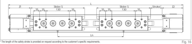
\* The length of the safety stroke is provided on request according to the customer's specific requirements.
