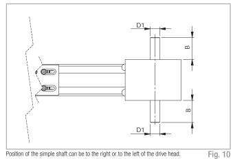
This head configuration is obtained by utilizing an assembly kit delivered as a separate accessory item.
