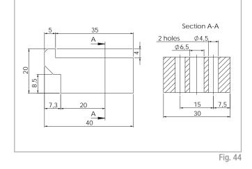
Fixing clamp (for all sizes except A100) for simple mounting of a linear axis on a mounting surface or for connecting two units with or without a connection plate (see p. US-70).
