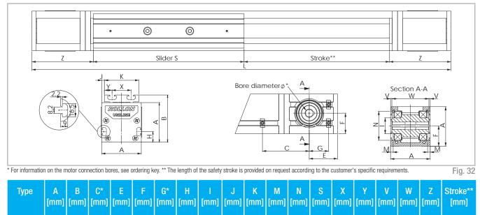
C55 55 71 67.5 50.5 27.5 32.5 15 Ø 24.9 1.5 52 2.35 Ø 47 200 28 12 0.5 54 108 1850 For the position of the T-nuts when using our motor adapter plates, see p. US-27ff Tab. 40 \*\* Maximum stroke for a single-piece guiding rail. For longer strokes, see tab. 45
