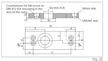
\* Area of plate needs to be cut if used for ED75 linear unit. (Adding 20 mm to total length of unit will render this modification unnecessary). Othewise it gets in contact with the outer rail. X = 20 mm; Y = 35 mm
