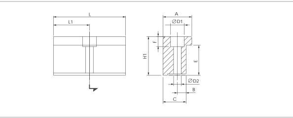
Anodised aluminum block for fixing the linear units through the side slots of the body
