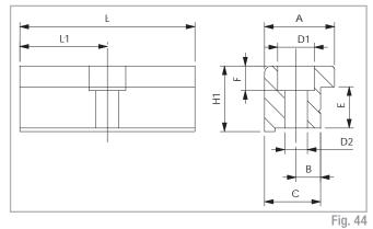
Anodised aluminum block for fixing the linear units through the side T-slots of the body.
