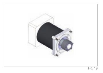
Assembly kit includes: srink disk; adapter plate; fixing hardware
