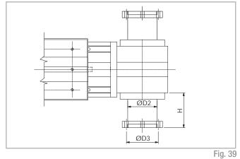
The series Robot linear units can be fitted with several different drive systems. In each case, the driving pulley is attached to the reduction gearshaft by means of a tapered coupling to ensure high accuracy over a long period of time.
