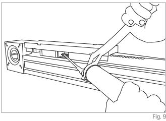
ball raceways under load. These lubrication reservoirs also considerably reduce the frequency of lubrication of the module. This system guarantees a long interval between maintenances: SP version: every 5000 km or 1 year of use, based on the value reached first. If a longer service life is required or in case of high dynamic or high loaded applications please contact our offices for further verification.
